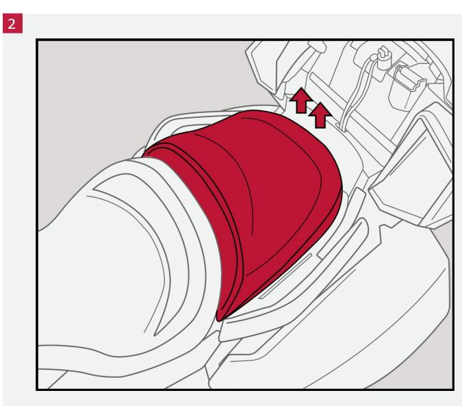
**F3 Only:** Release the passenger seat latch by pushing in on the key & turning it clockwise. Lift up the back of the seat to remove it.
