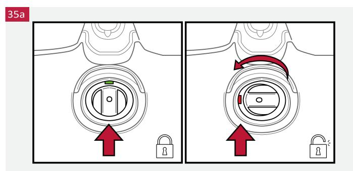
**RT Only:** With your cables hidden underneath the trunk area, you will unlatch the trunk compartment by turning the locking mechanism on the bottom surface of the trunk counter-clockwise 90 degrees.
