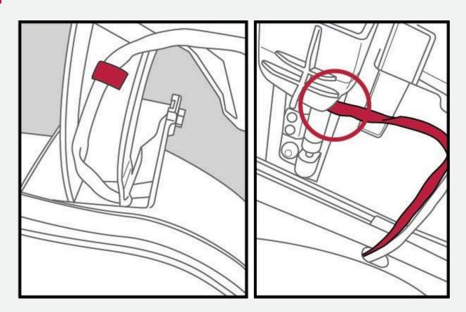
RT and F3: Feed your right light's cable along the trunk lid hinge and to the backrest panel area, similarly to the left side, but use the cutout by the trunk shock to feed your cable towards the passenger seat area.
