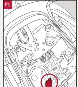
RT and F3: Locate the stock OEM tail harness location on the (left side for RTs) (right side for F3s) where the passenger seat is usually located.
