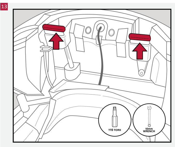
**RT and F3:** With the trunk lid closed, remove the trunk lid hinge pins using a 10MM WRENCH to hold the bolt head in place and a T-15 TORX to remove the screw at the opposite end.
