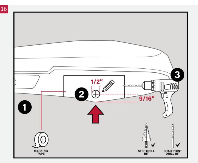
**RT and F3:** Flip the trunk lid so the finished surface faces up and the BRP logo faces you. We will start by focusing on the right-hand side of the trunk to begin the installation of the left side trunk light. Place a piece of MASKING TAPE on the trunk lid, as shown above.
