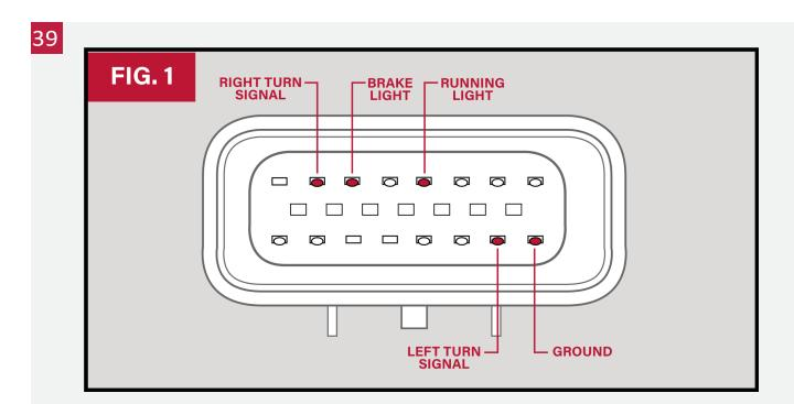
RT and F3: Unplug the stock OEM tail harness, utilize the T-TAP CONNECTORS provided, and T-tap into the wires coming off the pins labeled above.
