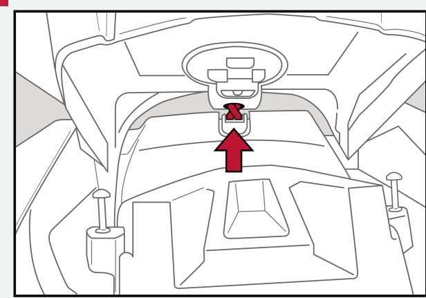
**RT Only:** With the trunk compartment tilted towards the front, locate the trunk light connectors and cables and feed them through the middle opening of the rear shroud panel towards the driver's seat.
