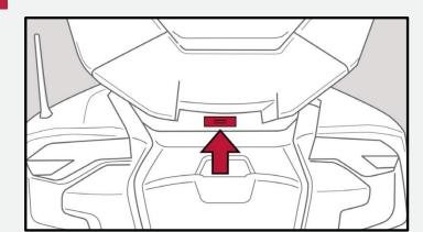
**RT Only:** The trunk compartment has a safety locking mechanism that, at this point, it will not allow you to tilt the trunk compartment forward any further; therefore, you will have to push the locking button seen above. This will enable you to fully unlock the trunk compartment and access the bottom side.
