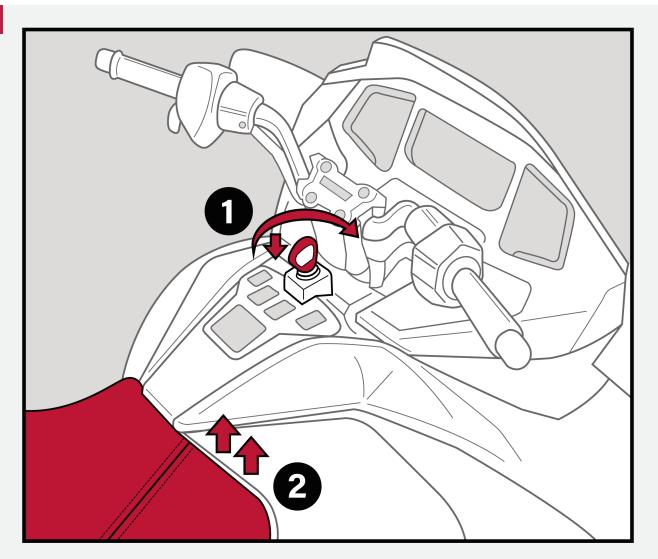
**RT Only:** Release the driver seat latch by pushing in on the key & turning it clockwise. Lift up the front of the driver seat to open it.
