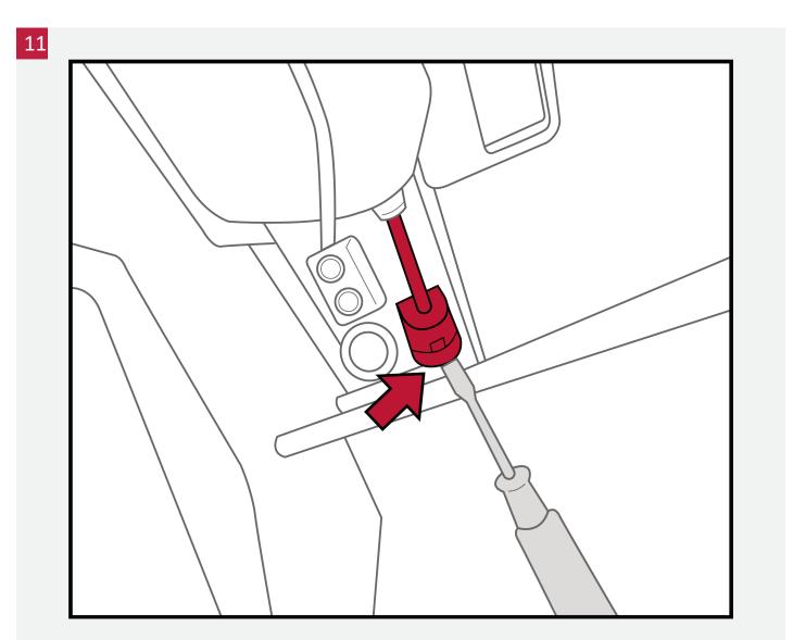
**RT and F3:** Using a FLAT SCREWDRIVER while supporting the lid, release (pry straight out) the metal clip securing the bottom of the trunk shock.
