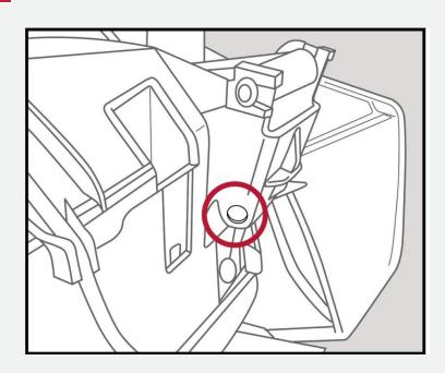
**RT and F3:** On the left side of the Spyder, drill a  $1/2^{"}$  hole on the section seen, this will allow you to feed you connector through the trunk lid's hinge onto the passenger's backrest area.
