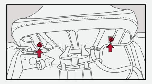
F3 Only: Using a 3/8" DRIVE RATCHET, 10MM SOCKET and a 6 INCH EXTENSION, remove the bolts holding the drivers seat.
