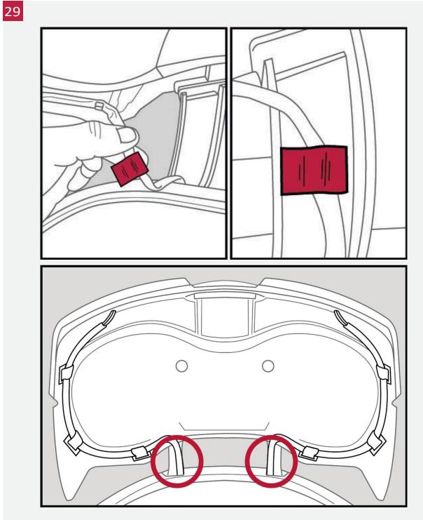
RT and F3: Place the modified ADHESIVE BACKED FLAT CABLE HOLDER to the left light's cable, peel away the backing and stick the holder to the hinge cavity.
