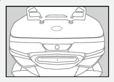
Some RTs and F3: If your Spyder has the stock OEM trunk lid fillers in the cavities where the FormFusion lights will be installed, remove them using fish line or any other item that will facilitate the removal process. After removing both inserts, remove the entire double sided tape residue left on the surface of the trunk.
