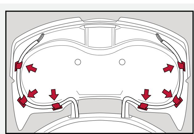
FLAT CABLE HOLDERS at the outer edge as desired.
