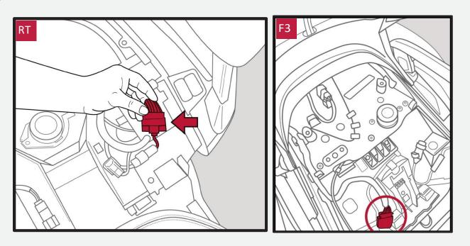
RT and F3: Locate the stock OEM tail harness location on the (left side for RTs) (right side for F3s) where the passenger seat is usually located.
