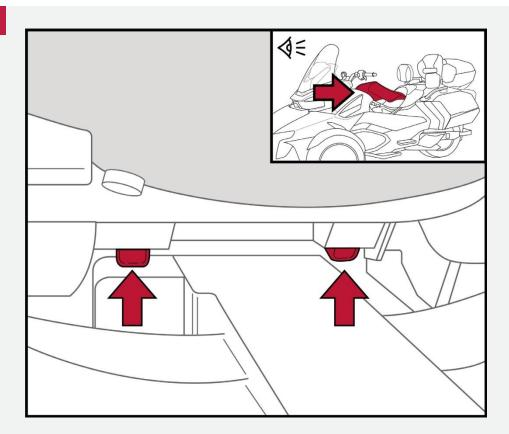
**RT Only:** Press the two tabs securing the front of the passenger seat from under the driver seat and lift up slightly to release (Located at the front bottom of the passenger seat under the driver seat).
