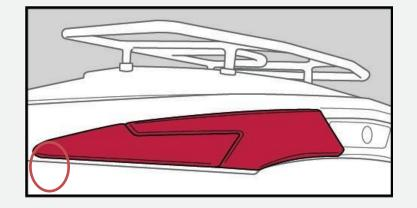
RT and F3: After confirming the appropriate fitment, wipe the surface where the trunk light will be mounted with the ADHESION PROMOTING WIPE provided. Once surface is dry, remove the backing tape from the left side trunk light and carefully press it into place on the trunk lid.
