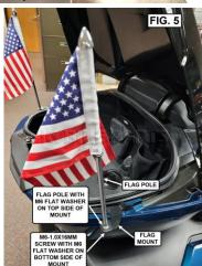
JSING THREADLOCK TO INSTALL HARDWARE WITH PLASTIC COMPONENTS, ONLY APPLY TO METAL COMPONENTS. IT IS CRITICAL THAT ANY EXCESS THREADLOCKER OR SPILLAGE IS CLEANED COMPLETELY FROM PLASTIC DIMPONENTS IMMEDIATELY BEFORE DRYING. A DAMP TOWEL OR RAG IS THE BEST WAY TO ACHIEVE THIS. IF EXCESS THREADLOCKER IS NOT CLEANED UP RIGHT AWAY, IT COULD LEAD TO DAMAGED PRODUCTS AND VOID WARRANTY.
