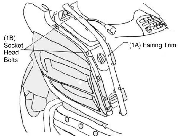
3. Install the left wind deflector (2A) by aligning the mounting brackets (2C) with the holes where the two fairing screws were removed. Two M5-0.8 x 16mm socket head bolts (1B) have been provided for installing each deflector. Use thread locking compound on the mounting screws. Do not over tighten.
